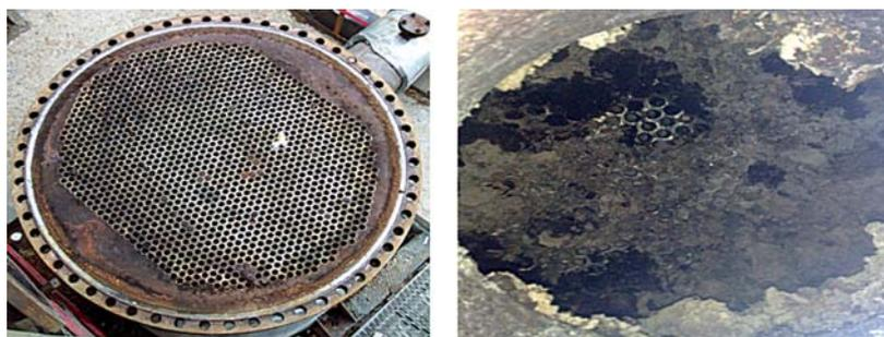
**Fig.1.** The surface of fractionator's trays in the case of using highly effective phenolic inhibitor and ineffective nitroxyl radicals
