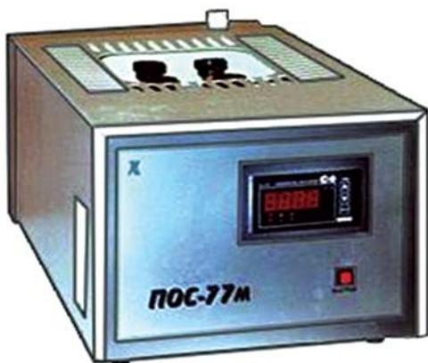
Fig.6. Special device "ПОО-77М" used for determination of polymer deposits
