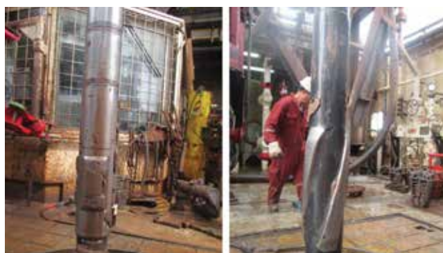
Figure 14. Clean BHA without adhering clay.
