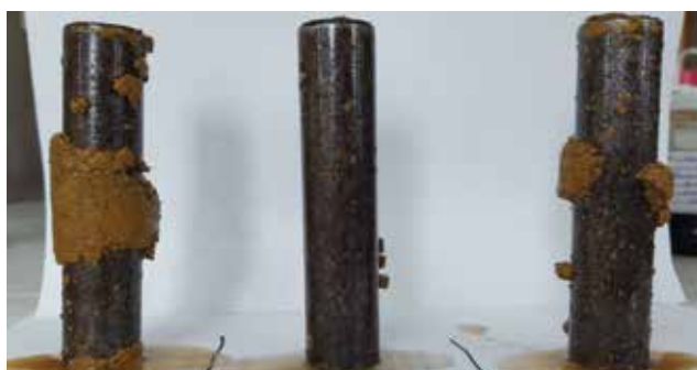
Figure 16. Anti-accretion test in KGAC Plus M1 DF system.
