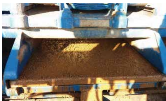
Figure 15. Drilled cuttings were well inhibited, dry and not sticky.
