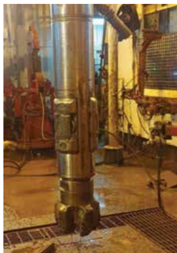
Figure 17. No bit-balling while drilling.
