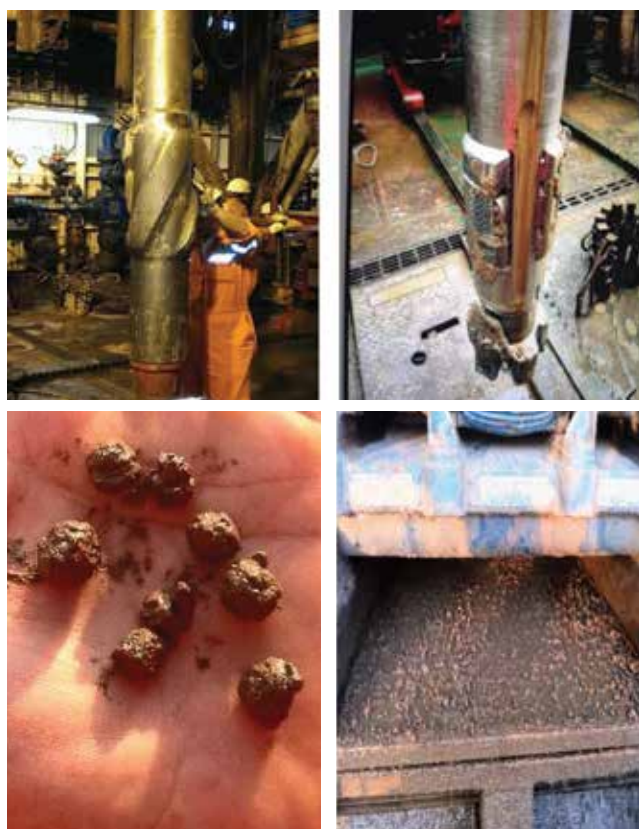
Figure 5. Field tests on Tam Dao 2 rig: There was very little clay adhesion on BHA pulled out, drilled cuttings were well inhibited, dry and nonsticky.
